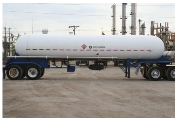
Figure 5: Typical Methyl Chloride trailer
