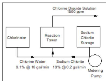
Figure 1. Chlorine Dioxide Generator
