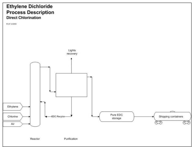
Figure 1: Direct Chlorination Reaction
