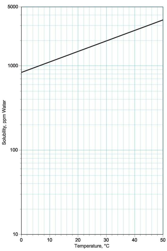
Figure 14: Solubility of Water in EDC Vs. Temperature
