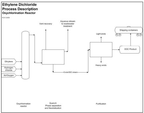
Figure 2: Oxychlorination Reaction
