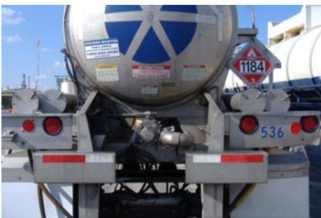
Figure 9: Truck Trailer Rear Product Outlet
