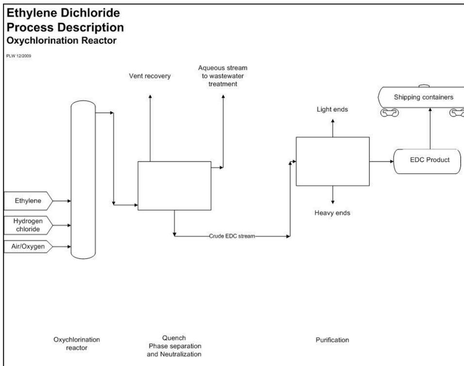
Figure 2: Oxychlorination Reaction
