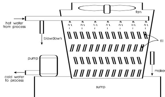
Figure 2 - Cooling Tower
