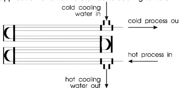
Figure 1. Heat Exchanger
